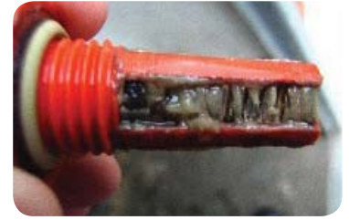
Nipple clogged with biofilm
