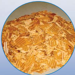
Lime stone on a heat exchanger
